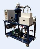
SFCV: Removes dirt plus water from oil
